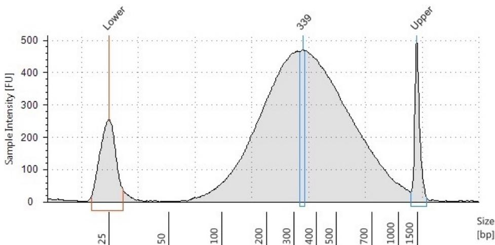
Electropherogram of sufficiently fragmented DNA sample, analyzed with Agilent HS D1000 ScreenTape.
